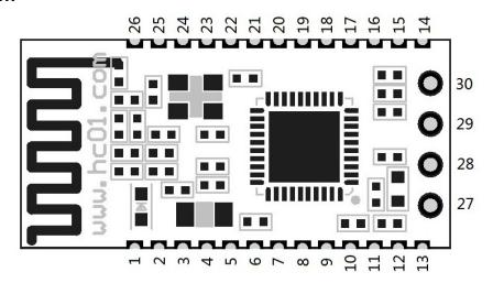
The HC-08 module has 30 pins, on board PCB antenna, pin specific definitions are listed in the following table:
