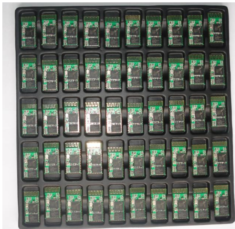
Figure 3 50 pieces chips in an anti-static blister package.
